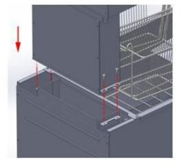
3. Slide the flue wrap over the flue. Secure it with self-tapping screws two on the back and two on the front using a 5/16" socket.
