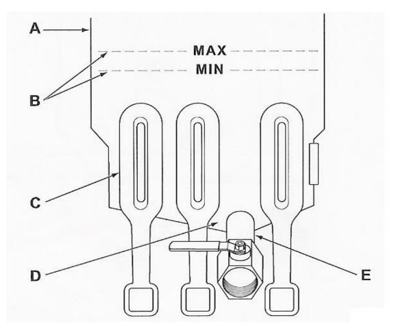
A Frying tank B Oil filling indicating line C Heating tube D Cold zone E Drain cock
